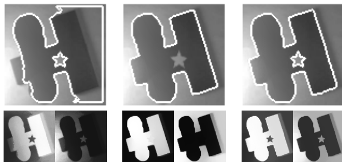
Fig. 5. Image segmentation affected by bias: Partition and ground states. left: CV-like region-based, center: GAC-like edge-based, and right: hybrid graph construction. Parameters: k = 2 , q = 2 , \alpha = 2 , 60 edges per vertex, \epsilon = 0.001 , p = 0.1 , \lambda = 250 ; hybrid sampling radius r = 8 .
