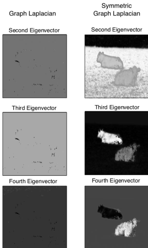
**Fig. 2.1** *Eigenfunctions from the graph Laplacian obtained from the cow image in section 4.3. The left column shows eigenvectors of the unnormalized Laplacian  $L$  as in (2.4). The right column shows eigenvectors of the symmetric graph Laplacian  $L_s$  as defined in (2.6).*
