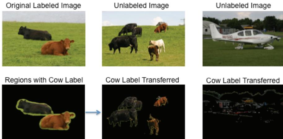
**Fig. 4.7** This figure uses the same labeled image as in Figure 4.6 and tries to classify similar features in additional images. We include one image with a white colored cow and another image with clutter and no cows. Original images in the top row are from the Microsoft Research Cambridge Object Recognition Image Database [2] (copyright © Microsoft Corporation). These images were modified to produce the images in the bottom row (8 April 2012).
