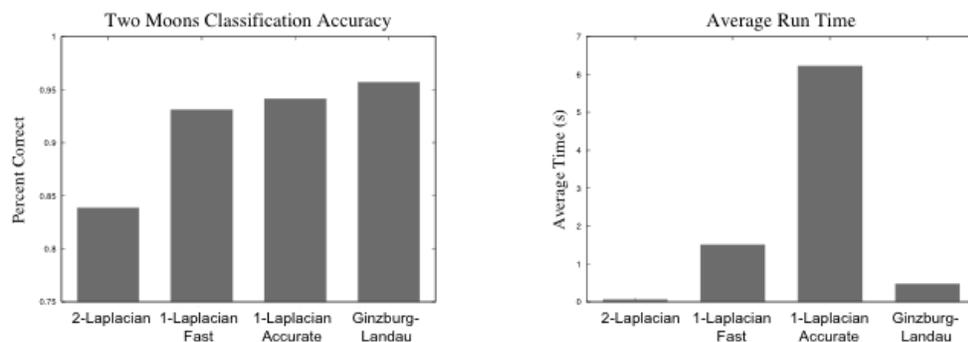
**Fig. 4.5** *The accuracy of the GL unsupervised segmentation procedure presented in this paper is compared with spectral clustering and the 1-Laplacian code of Hein and Bühler [42]. These two graphs were created using 100 runs of the Two Moons dataset and averaging the results.*
