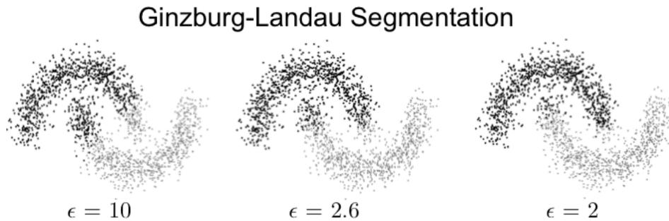
**Fig. 4.3** The parameter  $\epsilon$  determines a scale for the GL energy functional. A more accurate segmentation is obtained as the  $\epsilon$  scale parameter decreases. The percentage of correct classification was 82.85%, 90.75%, and 94.55% for  $\epsilon = 10, 2.6,$  and  $2,$  respectively.
