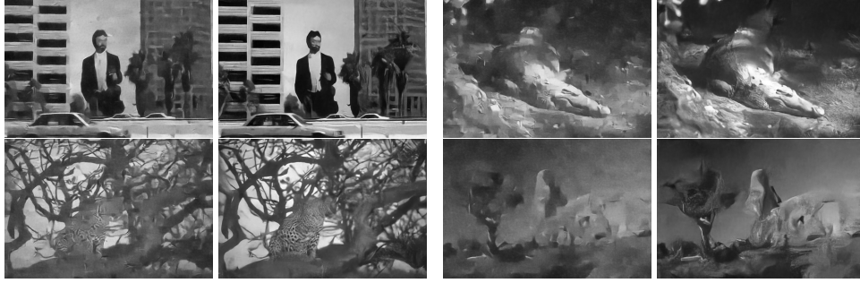
Figure 8: Denoising results of different restoration unit structure designs. Left images are produced by the AR-CNN-like unit. Right images are produced by our proposed minimal U-Net style network.
