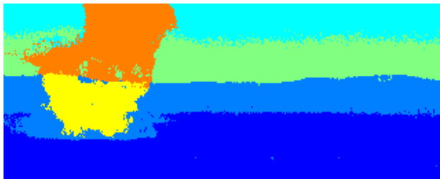
FIGURE 4. Segmentation of a hyperspectral video using graph MCF. The gas plume is clearly represented in the yellow and orange pixels. The two bottom blue classes are the ground, and the other two are the sky. This image is frame 3 of 7.
