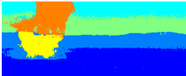
Figure 4.3: Segmentation of a hyperspectral video using graph MCF. The gas plume is clearly represented in the yellow and orange pixels. The two bottom blue classes are the ground, and the other two are the sky. This image is frame 3 of 7.
