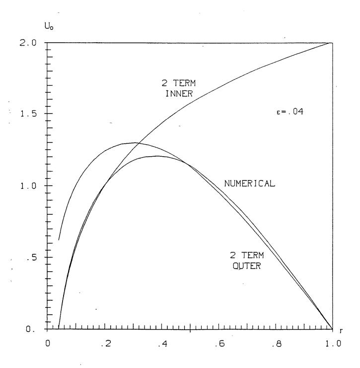
Figure 5 Comparison of one and two term composite approximations of u(r;  $\epsilon$ ) with accurate numerical solution for  $\epsilon$  =0.04 at the limit point  $\lambda_o(\epsilon)$
