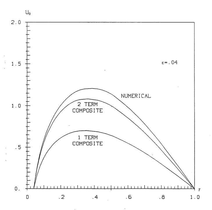
Figure 6 Comparison of one and two term composite expansions of  $u(r; \epsilon)$  with accurate numerical solution for  $\epsilon$  =0.001 at the limit point  $\lambda_o(\epsilon)$
