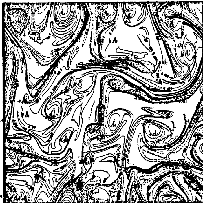
Figure 9 Contour plots of the vorticity for smooth random initial data, \nu = 2 \times 10^{-5} , N = 256 .
