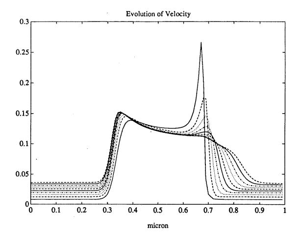
Fig 16: Evolution of velocity  $v(t)=t, \ Time=20, \frac{\Delta t}{\Delta x}=.1, \Delta x=.01$
