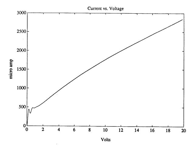
Fig 12: Current vs. Voltage  $v(t)=t, \ Time=20, \frac{\Delta t}{\Delta x}=.1, \Delta x=.01$
