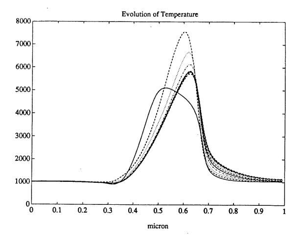
Fig 19: evolution of temperature  $v(t)=2H(t),\ Time=3, \frac{\Delta t}{\Delta x}=.1, \Delta x=.01, T_0=1000K$
