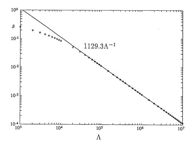
Figure 1(b). Growth rate, s, as a function of  $\Lambda$  in a log-log plot for a case in which there is no critical level in the layer:  $k_x = k_y = 1$ ,  $q = \frac{1}{2}\pi$  and R = 8.5 (<  $R_c$ ).
