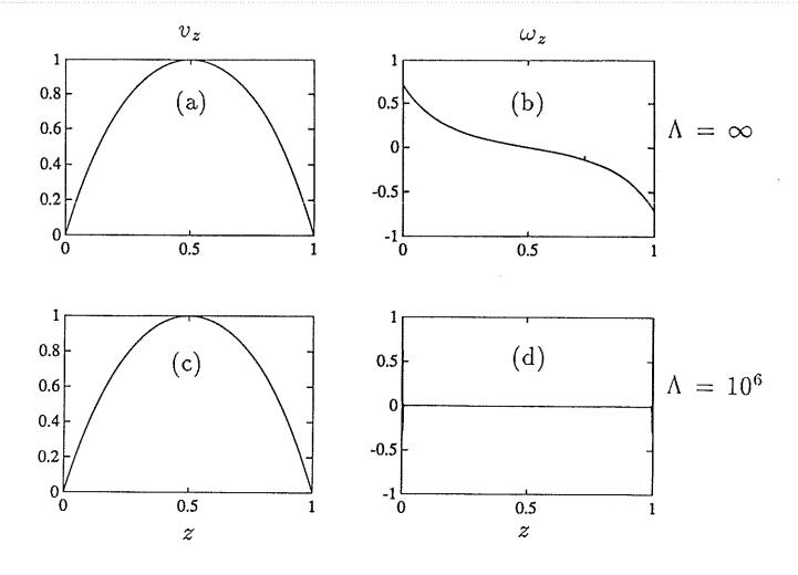
Figures 3. Comparisons between eigenfunctions for stable ideal modes ( $\Lambda=\infty$ ) [panels (a) and (b)], and those for the corresponding resistive instabilities for large  $\Lambda$  [panels (c) and (d)]. There is no critical level in the layer; in all cases  $k_x=k_y=1, q=\frac{1}{2}\pi$ , and R=8.5; in (c) and (d),  $\Lambda=10^6$ . The velocity perturbation,  $v_z$ , is shown in panels (a) and (c) and the vorticity perturbation,  $\omega_z$ , in panels (b) and (d).
