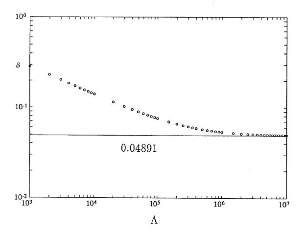
Figure 1(a). Growth rate, s, as a function of  $\Lambda$  in a log-log plot for a case in which there is no critical level in the layer:  $k_x = k_y = 1$ ,  $q = \frac{1}{2}\pi$  and R = 8.6 (>  $R_c$ ).
