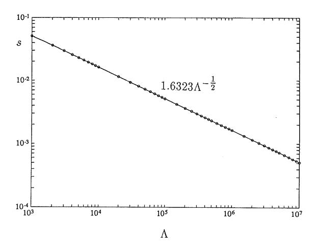
Figure 5(b). Growth rate, s, as a function of  $\Lambda$  in a log-log plot for a case in which there is no critical level in the layer:  $k_x = k_y = 4$ ,  $q = \frac{3}{2}\pi$  and R = 1 (<  $R_c$ ).
