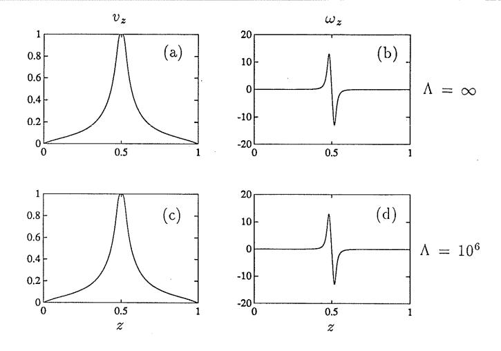
Figures 6. Comparisons between eigenfunctions for ideal instabilities ( $\Lambda = \infty$ ) [panels (a) and (b)], and those for the corresponding instabilities for large  $\Lambda$  [panels (c) and (d)]. There is one critical level in the layer; in all cases  $k_x = k_y = 4$ ,  $q = \frac{3}{2}\pi$ , and R = 12; in (c) and (d),  $\Lambda = 10^6$ . The velocity perturbation,  $v_z$ , is shown in panels (a) and (c) and the vorticity perturbation,  $\omega_z$ , in panels (b) and (d).
