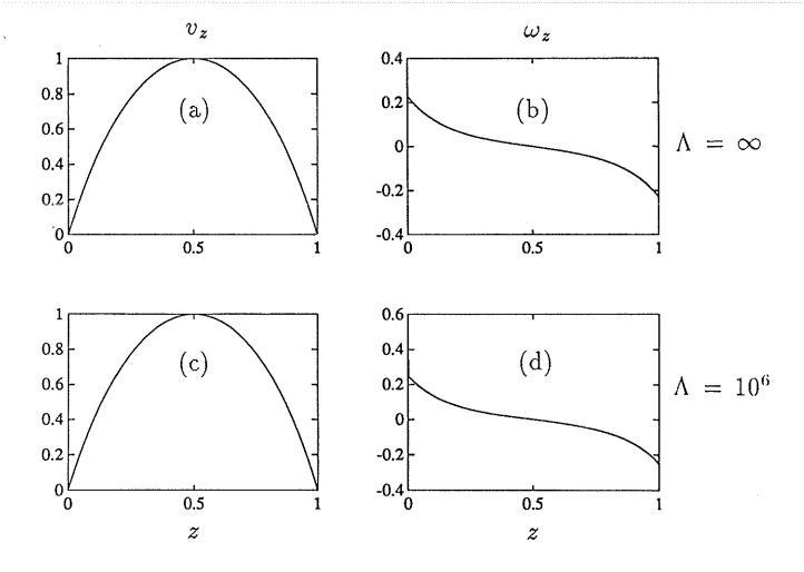
Figures 2. Comparisons between eigenfunctions for ideal instabilities ( $\Lambda=\infty$ ) [panels (a) and (b)], and those for the corresponding instabilities for large  $\Lambda$  [panels (c) and (d)]. There is no critical level in the layer; in all cases  $k_x=k_y=1, q=\frac{1}{2}\pi$ , and R=8.6; in panels (c) and (d),  $\Lambda=10^6$ . The velocity perturbation,  $v_z$ , is shown in panels (a) and (c) and the vorticity perturbation,  $\omega_z$ , in panels (b) and (d).
