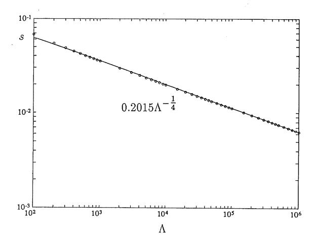
Figure 8(a). Log-log plot of the growth rate, s, of resistive instabilities as a functions of  $\Lambda$  for fast g-modes when there is one critical level in the layer:  $q = \frac{3}{2}\pi$  and  $R = 0.5(< R_c)$ . In the case shown,  $k_x = k_y = \Lambda^{1/4}$ .
