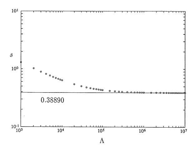
Figure 5(a). Growth rate, s, as a function of  $\Lambda$  in a log-log plot for a case in which there is one critical level in the layer:  $k_x = k_y = 4$ ,  $q = \frac{3}{2}\pi$  and R = 12 (>  $R_c$ ).
