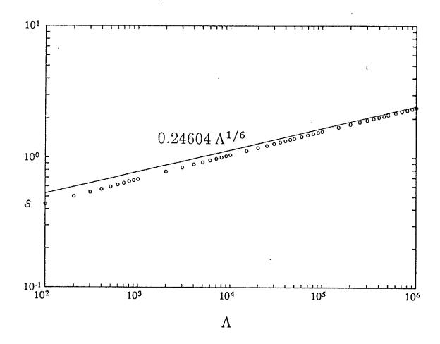
Figure 8(c). Log-log plot of the growth rate, s, of resistive instabilities as a functions of  $\Lambda$  for fast g-modes when there is one critical level in the layer:  $q = \frac{3}{2}\pi$  and  $R = 0.5(< R_c)$ . In the case shown,  $k_x = k_y = \Lambda^{3/4}$ .
