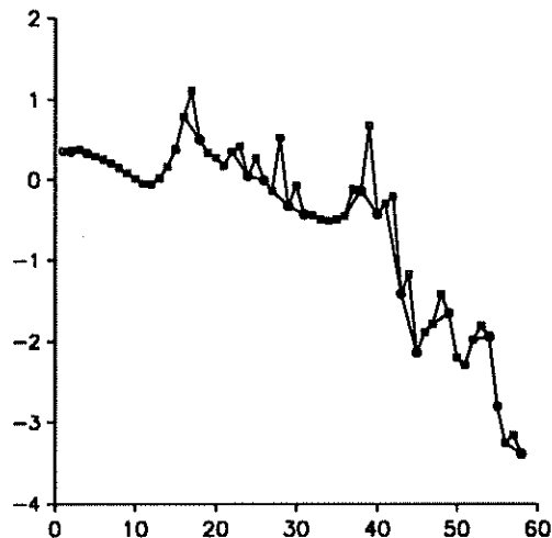
FIG. 1. Convergence history e_k v. k for \beta = 10 . BCG iterates are open boxes, CSBCG iterates are filled boxes ( 1 \times 1 steps) and filled circles ( 2 \times 2 steps).
