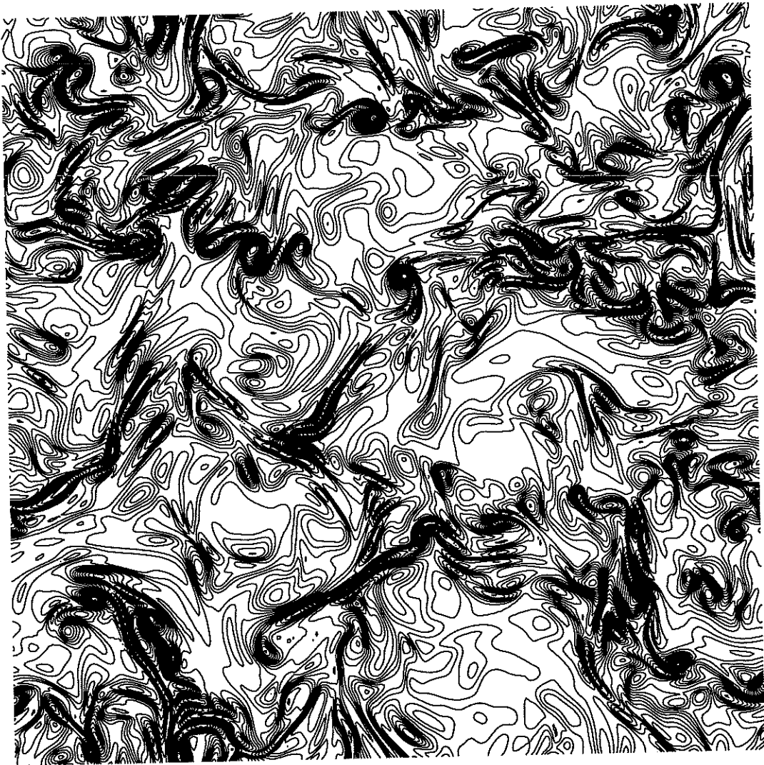
Figure 8: Contour plots of the y component of the vorticity, base-run-E for y = y_{60} at t = t_0 = 6.0 , (\min, \max) = (-41.8, 79.8) , contour spacing: 2
