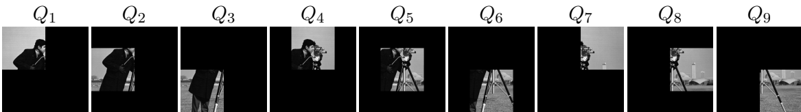
Figure 4: Scanning positions generated by the illumination windows described in Section 4.1.2. For the small problem where n_1 = n_2 = 512 (Section 4.1.1), each illumination window Q_i has size 256 \times 256 and shifts 128 pixels at a time. Similarly, for the large-scale problem where n_1 = n_2 = 16384 (Section 4.1.3, each illumination window Q_i has size 8192 \times 8192 and shifts 4096 pixels at a time. In both setups, there is a 50% overlap between consecutive probes.
