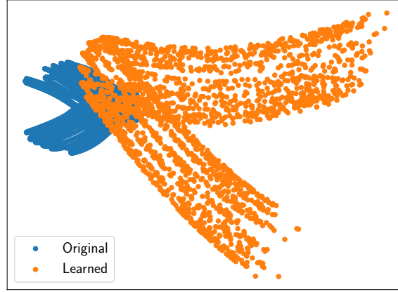
Figure 3: The ground truth and learned latent ( \mathbf{p} -variable) dynamics look very similar, but differ roughly by a rigid body transformation and rescaling. This indicates that the latent space does carry information for the synthetic data, i.e., LDDMD has an interpretable latent space.
